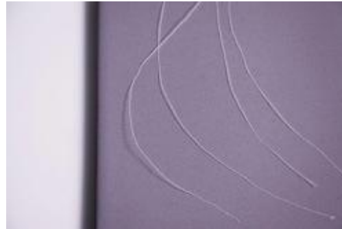
Fibre yarn directly from cellulose pulp or nanocellulose
