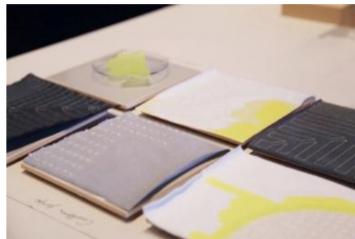
New textiles structures by 3D direct write printing of thermoplastic cellulose on cellulose matrix
