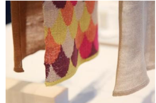
Textiles from recycled paper and from lignin containing materials with intrinsic lignin derived color
