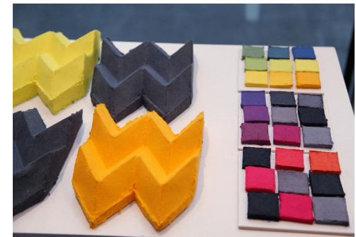
Designed 3D foams from cellulose fibres
