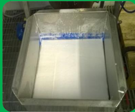
Forming mould with fibre foam
