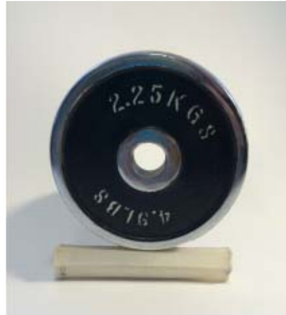
Hexagonal tube with 2,25 kg weight: CNF, Masuko3, pine (VTT), Dimensions: weight 9,2 g, length 150 mm, thickness of CNF ~ 0,53 mm
