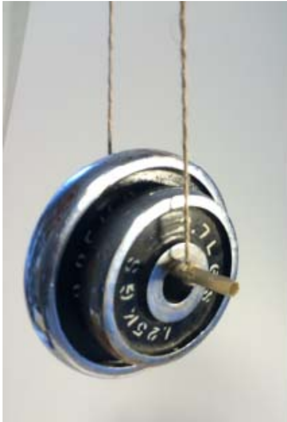
Tube with 4,75 kg weights: Material CNF, Masuko3, pine (VTT) Dimensions: weight 3,2 g; length 130 mm, diameter ~9,2 mm, thickness of CNF ~0,73 mm
