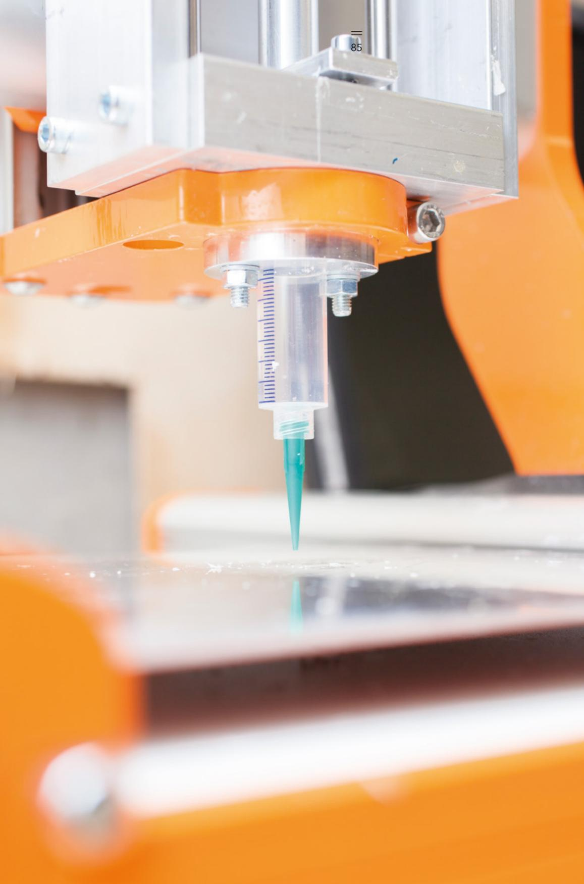
**FIGURE 72** Extruder prototype for 3D printing non-thermoplastic cellulosic materials. Designed and constructed by Pyry Kärki and Ville Klar.
