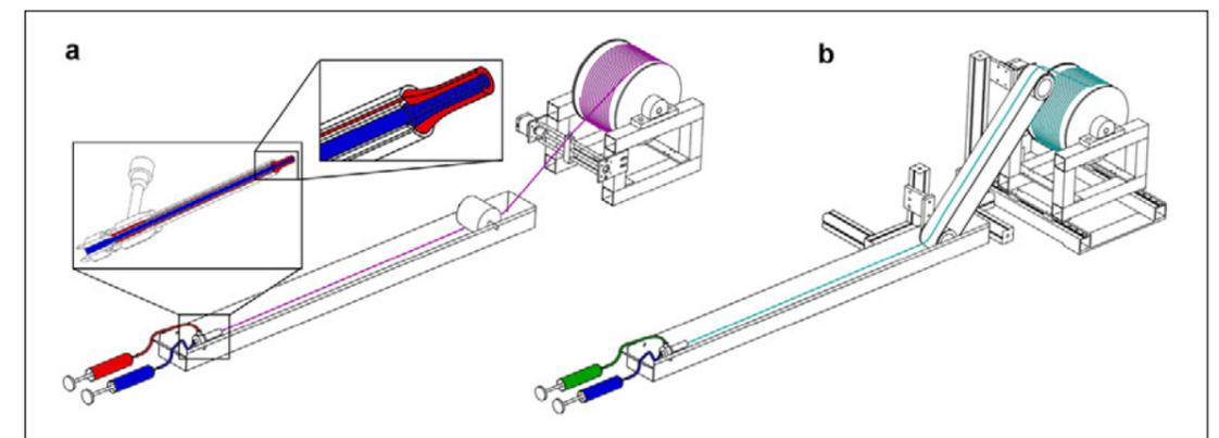
**FIGURE 67** Schematic views of spinning lines without (a) and with (b) a conveyor belt.
