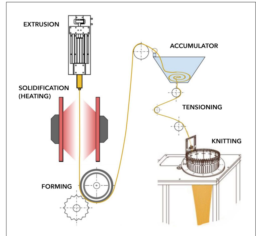
**FIGURE 83** Illustration of a combined spinning and knitting process.
