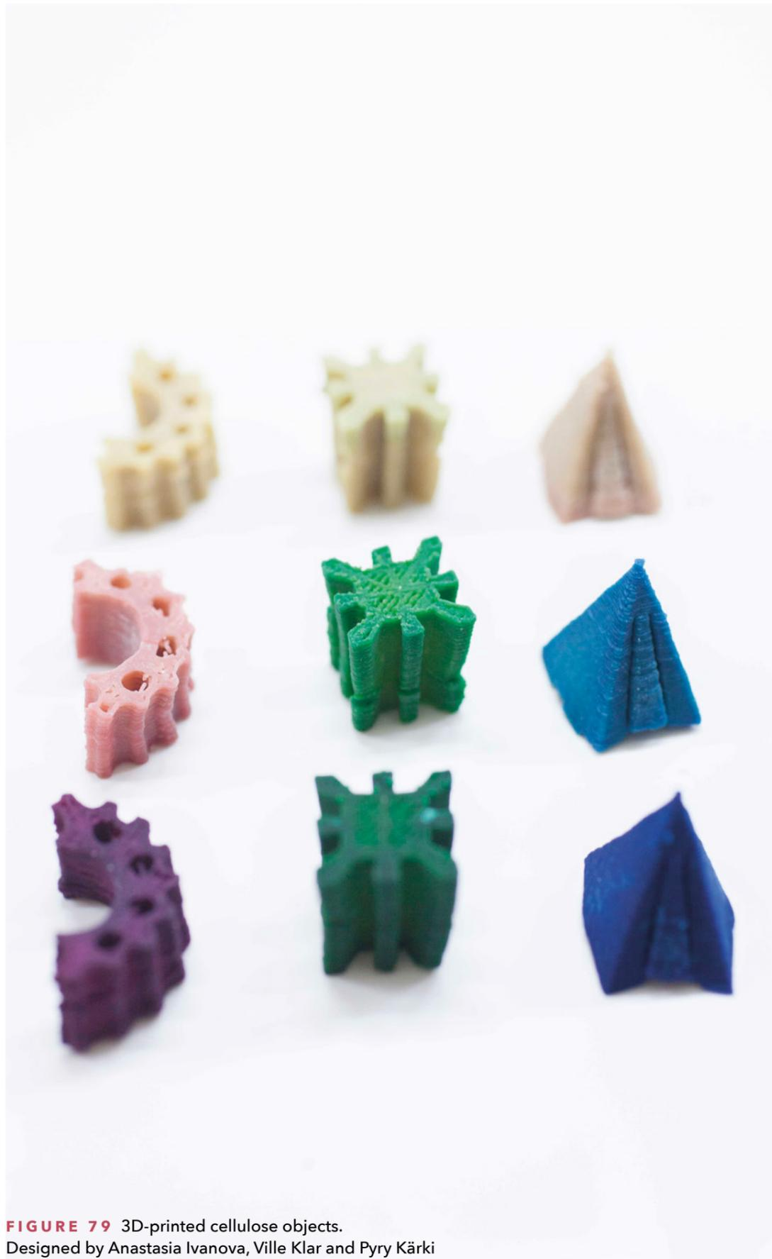
**FIGURE 79** 3D-printed cellulose objects.
