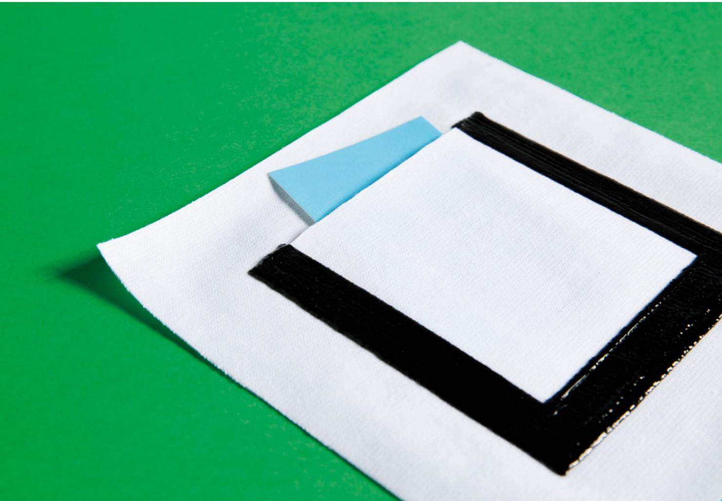
**FIGURE 77** Structures printed using cellulose dissolved in ionic liquid could be used for smocking effects. Design by Pauliina Varis and Ilona Damski, 2016-2017
