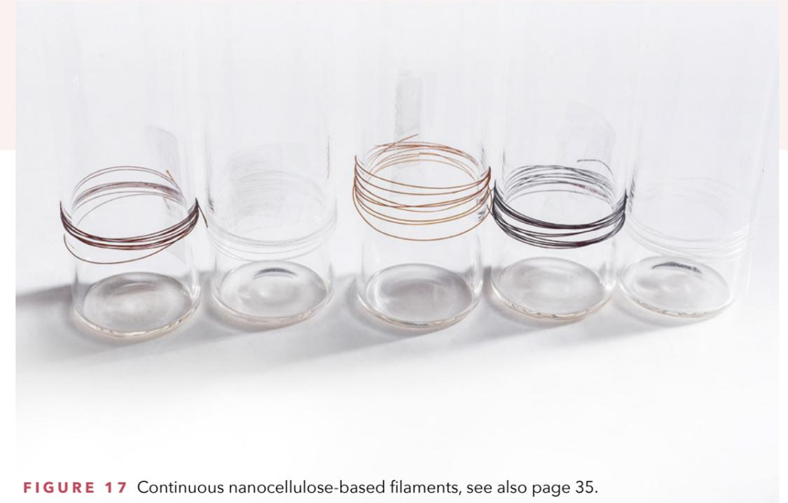
FIGURE 17 Continuous nanocellulose-based filaments, see also page 35.
