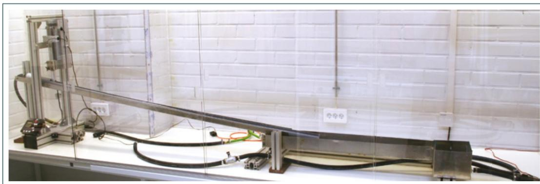
**FIGURE 68** Prototype inclined channel spinning line. Photo: Ville Klar.
