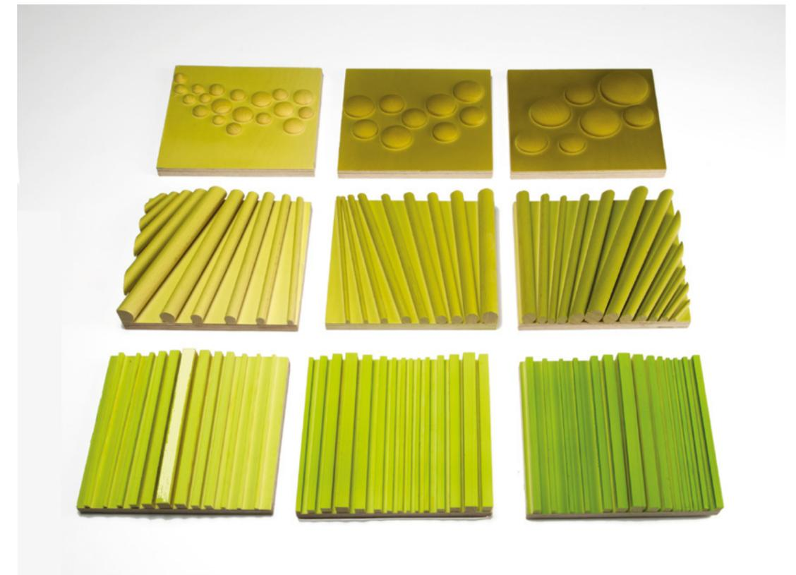
**FIGURE 61** Wooden reliefs painted with coloured nanocellulose.
