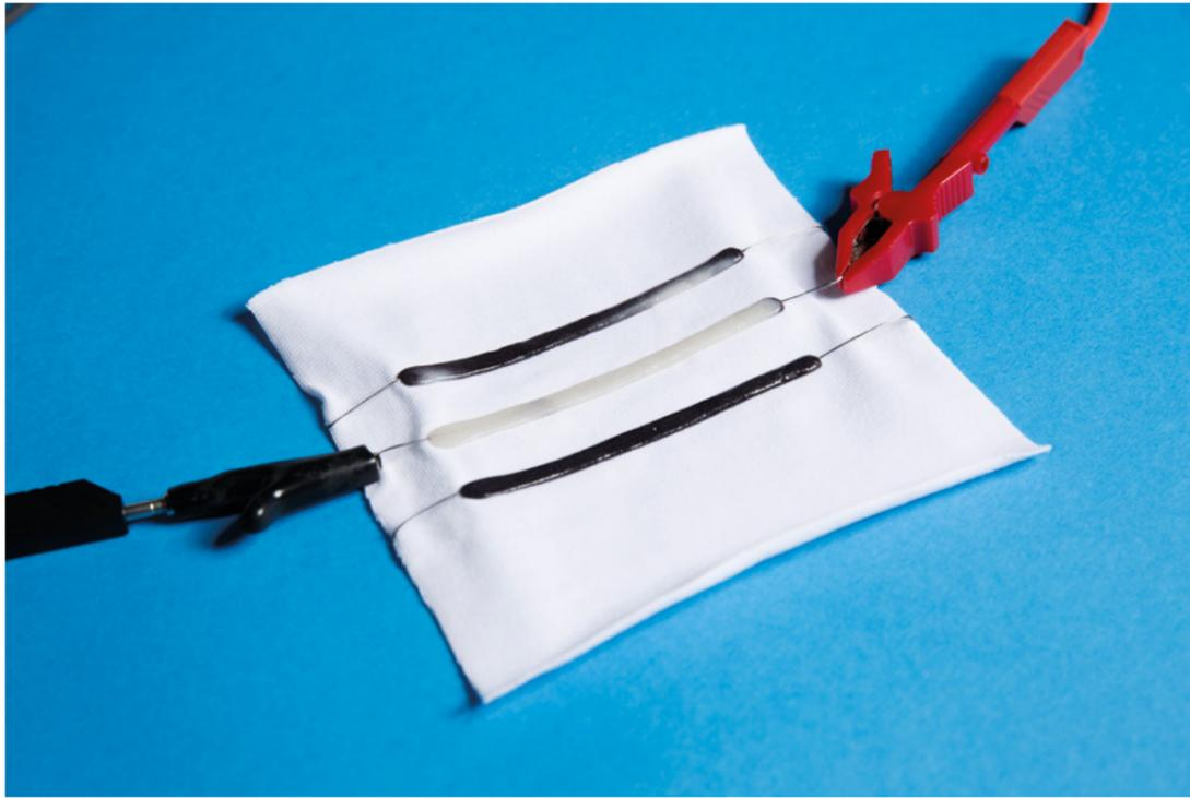
**FIGURES 75, 76** 3D-printed textiles, functional prototypes. Designed by Pauliina Varis. Above: A thermoresponsive prototype utilising thermochromic powder mixed with APC solution. A conductive metal yarn is embedded into the print. When current passes through the wire, the produced heat changes the color of the printed tag on the fabric. Below: Printed seam material (coloured APC) replacing stitches in the pocket.
