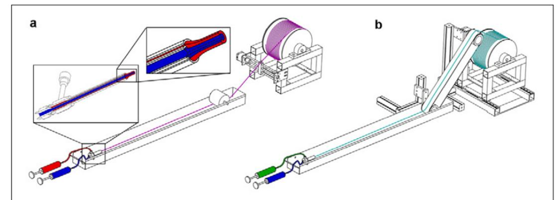
**FIGURE 67** Schematic views of spinning lines without (a) and with (b) a conveyor belt.
