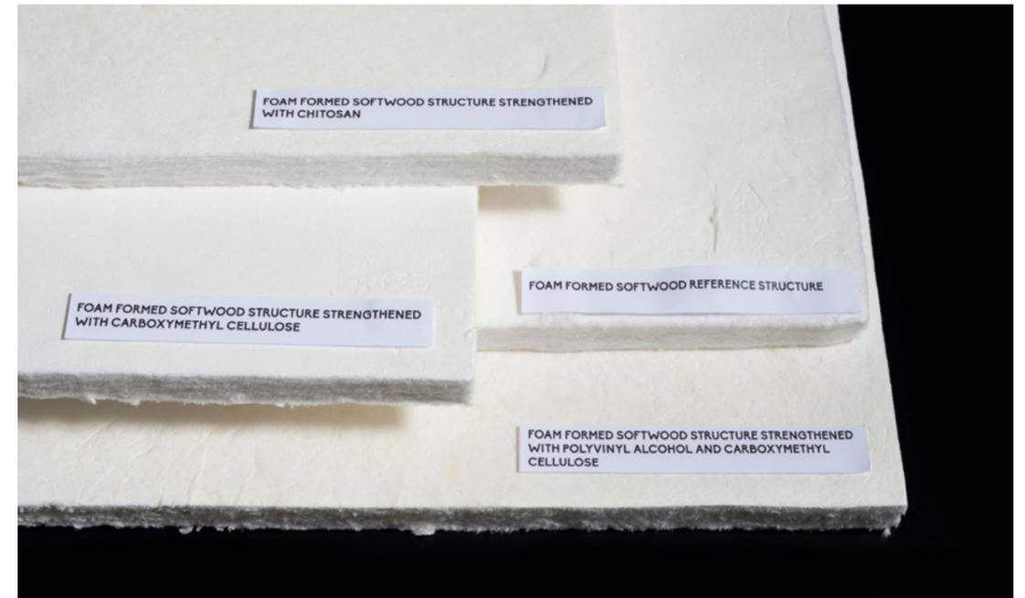
**FIGURE 50** Researching the strengthening of foam panels.
