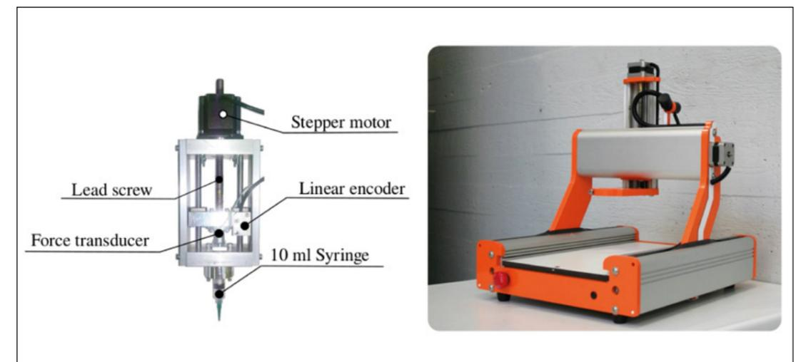
**FIGURE 71** Syringe extruder prototype and 3D-printer frame. Photo by Ville Klar.
