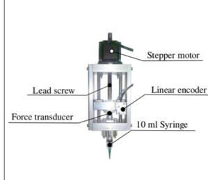
FIGURE 71 Syringe extruder prototype and 3D-printer frame. Photo by Ville Klar.
