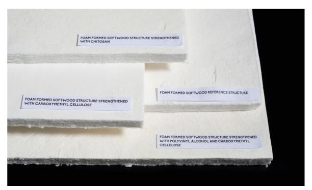
**FIGURE 50** Researching the strengthening of foam panels.
