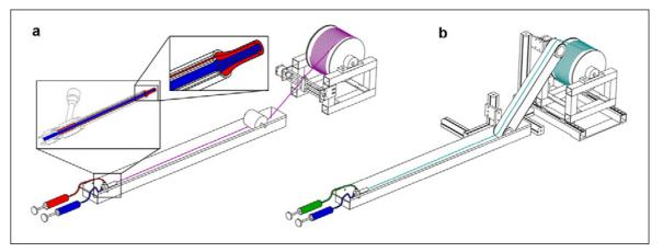
FIGURE 67 Schematic views of spinning lines without (a) and with (b) a conveyor belt.
