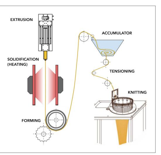
FIGURE 83 Illustration of a combined spinning and knitting process.
