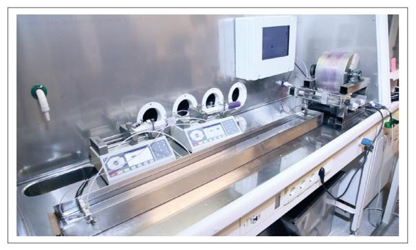
FIGURE 66 Photograph of coaxial spinning line prototype. Photo by Ville Klar.
