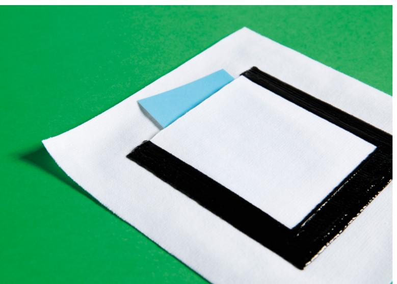
printed using cellulose dissolved in ionic liquid could be used for smocking effects. Design by Pauliina Varis and Ilona Damski, 2016-2017
