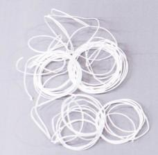
increased from 15.5  $\pm$  1.7 GPa to 21.3  $\pm$  5.5 GPa, while elongation at break decreases from  $6.9 \pm 0.9$  % to  $2.8 \pm 0.5$  %. However, the pretreated filaments retain less than 1% of their strength in wet conditions, and untreated filaments retain close to 2%. Wet strength can be increased above 80% of dry strength via UV-crosslinking.
