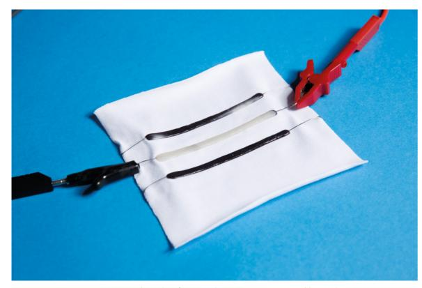
FIGURES 75, 76 3D-printed textiles, functional prototypes. Designed by Pauliina Varis. Above: A thermoresponsive prototype utilising thermocromic powder mixed with APC solution. A conductive metal yarn is embedded into the print. When current passes through the wire, the produced heat changes the color of the printed tag on the fabric. Below: Printed seam material (coloured APC) replacing stitches in the pocket.
